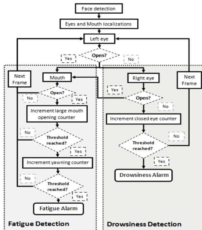
Figure 3. Driver's fatigue and drowsiness respectively detection system
