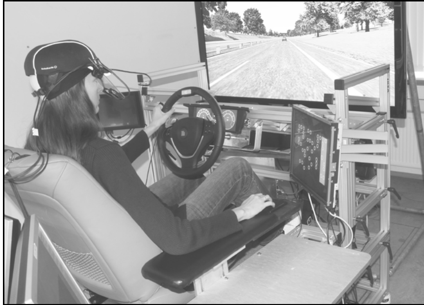
Figure 1. Experimental setup: Participant is performing driving task, head-mounted detection response task and SuRT at the same time
