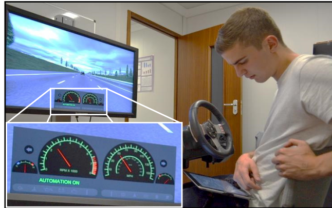
Figure 1. Driving simulator set-up. The central display unit (inset) indicated automation status. A 'beep' tone alerted drivers to changes in automation status
