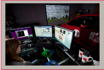
The AgeLab simulator running STISIM Drive v.2.08.02 on a 8' by 6' projection screen providing approximately a 40 degree view of a virtual world at 1024 x 768 pixel resolution. Primary task instructions and auditory stimuli are all presented under program control for consistency of presentation.
