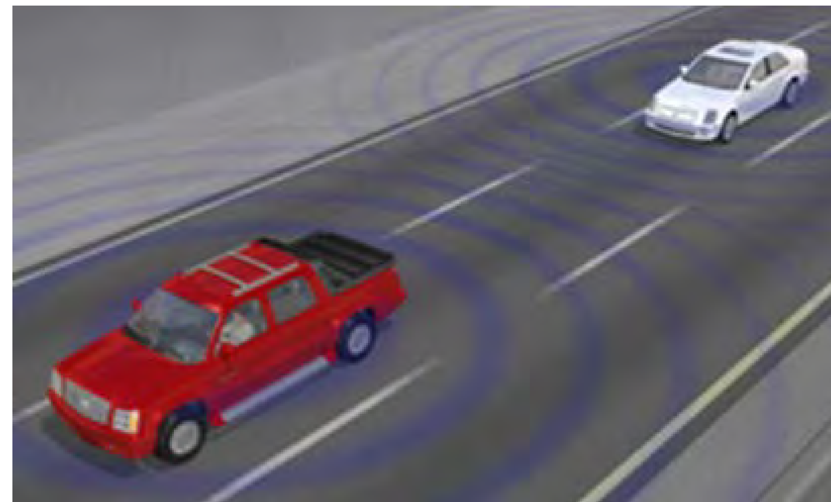
CACC uses DSRC*, allowing vehicles and infrastructure to communicate directly.
