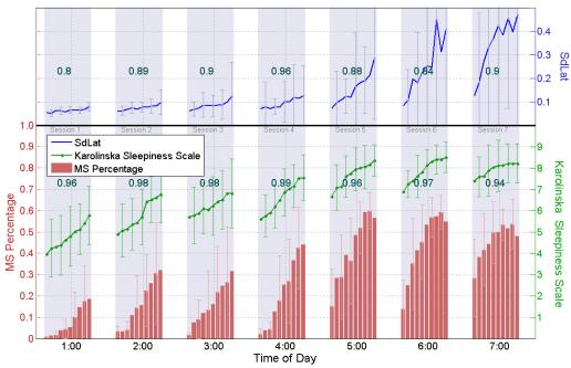
Figure 3.Mean and standard deviation of MS percentage (red), subjective sleepiness (green), and standard deviation of lateral position of the vehicle(blue). Averaging interval was 4 min. Strong correlations between both objective and subjective measures are indicated by Pearson's coefficients
