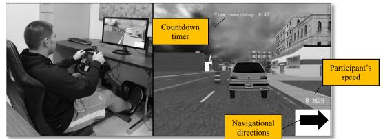
Figure 1. Configurations of driving simulator and scenarios - left image is the driving simulator apparatus and right image is an example of a slow-moving lead vehicle frustrating event. The countdown clock, driver's current speed in miles per hour, and the navigational directions are depicted
