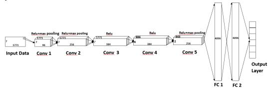
Figure 3. Architecture of modified AlexNet
