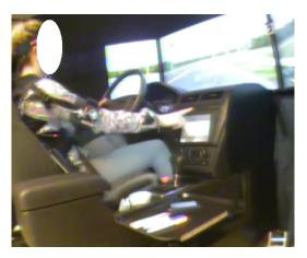
Figure 1. Experiment Setup. The figure shows the participant is using the navigation panel while driving on highway scenario with right wrist kinematics tracked by an IMU sensor
