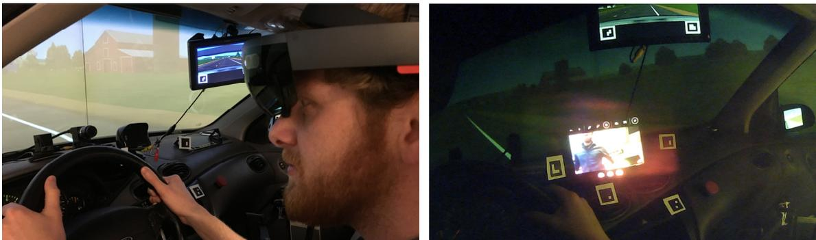
Figure 1. Participants operated a simulated vehicle and wore a HoloLens augmented reality (AR) device (left). HoloLens projected an AR Skype window for communication with a remote conversant (right).
