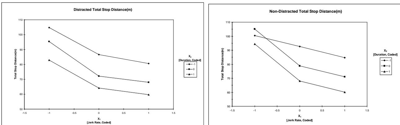
Figure 2. Total stopping distance as function of pulse braking display jerk rate and duration for distracted and non-distracted conditions.
