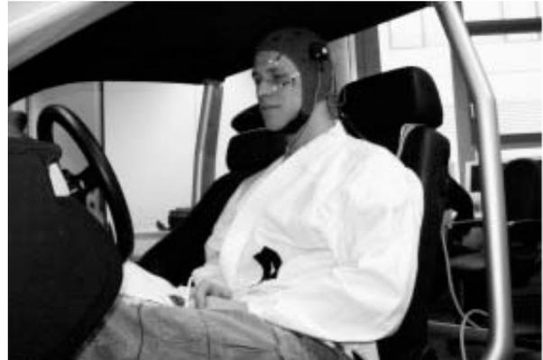
**Figure 1.** Instrumented driver in the simulator.
